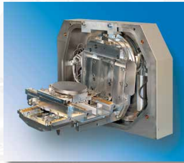
5-axes-manipulator for scanning electron microscopes SEM (X-, Y- and R-axes driven by Piezo-motors)
