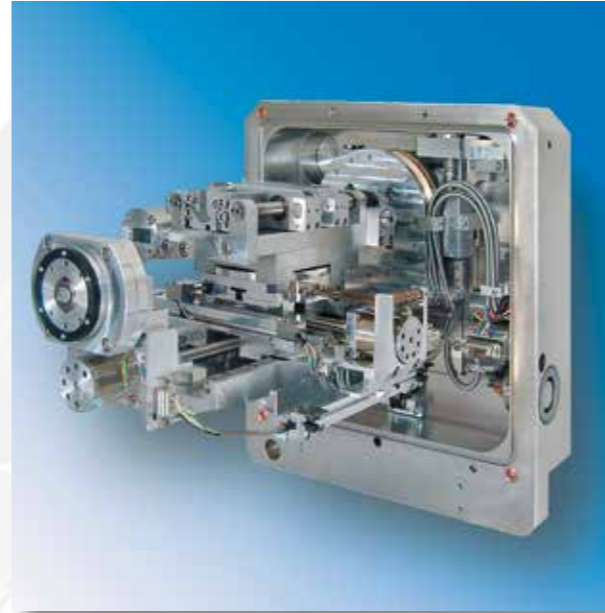
Module for heating- and tensile tests assembled on top of a 5-axes-manipulator for SEM
